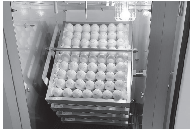
Figure 7 : The mostly used machine in this surveillance was egg incubator (監視業務で最も使用された機械は孵卵器でした)
